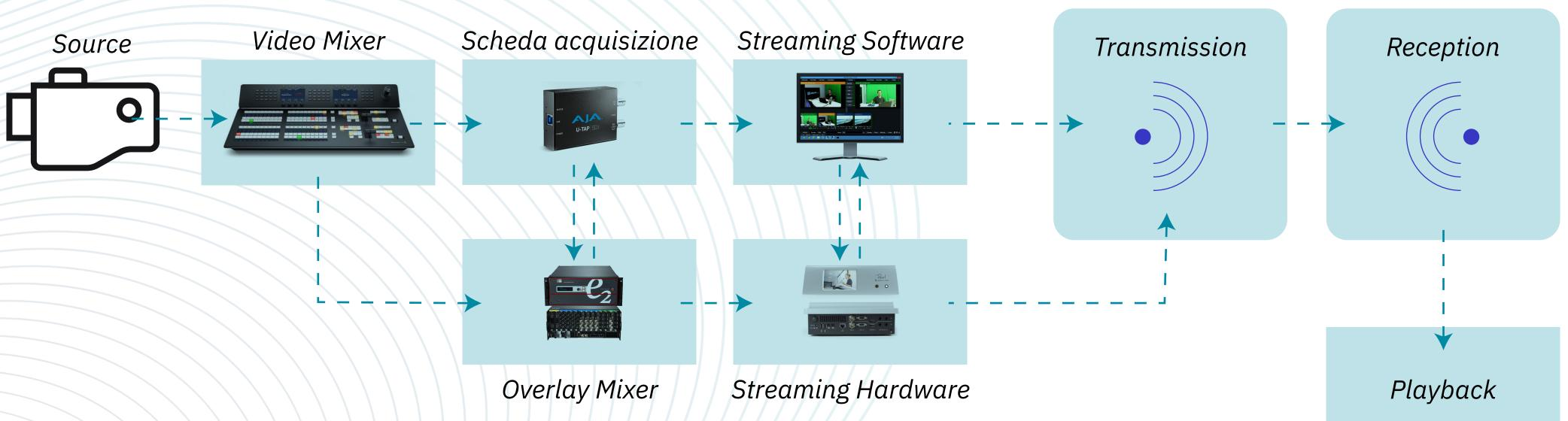
The video signal is captured in high definition and will be compressed to reduce bandwidth usage, introducing additional delay to the signal processing.
